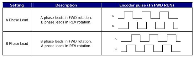
If you set "Enc Err Chk" of PAR\_12 to "Yes", when there is disconnection or misconnection of encoder, encoder error is detected and show the encoder abnormity sign. In the case of open collector method of encoder, it isn't possible to detect encoder error. So set PAR-12 to "No".
