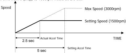
Setting example 2 If FUN\_33 is set to 'Ref Speed' and speed command and acceleration time is set to 1500rpm and 5 seconds, respectively, it takes 5 seconds to accelerate from the standstill to 1500rpm.
