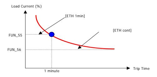
The motor protection is possible by calculating and accumulating 12t even in load variation and frequent run/stop.
