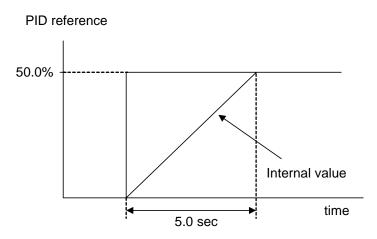
Tension Command where Ramp Time is applied
