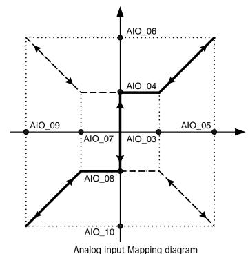
AIO\_03 Ai1 In X1 and AIO\_05 Ai1 In X2 are for setting the allowed range of voltage of current that is fed into analog input terminal, so generally you can set AIO\_03 Ai1 In X1 as 0[%], and AIO\_05 Ai1 In X2 as 100[%]. But, the analog input device make happen Chattering around 0[%], you can adjust the set value of AIO\_03 Ai1 In X1 up to the level of escaping the Chattering.
