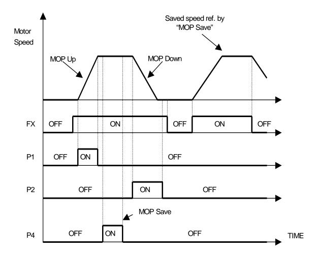
(MOP Clear setting example 3) To clear the saved speed by MOP Save function, use "MOP Clear ON/OFF". If MOP Clear is ON during running, the inverter decelerates its speed to zero speed. If MOP is ON during stop, this function resets the speed reference to "0".
