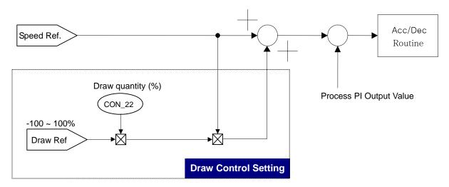
One of the multi-function analog input is set to the draw command ranging from -100% to 100% and the speed command multiplied by Draw quantity is added up to the speed command (Speed Ref) to obtain the final speed command.
