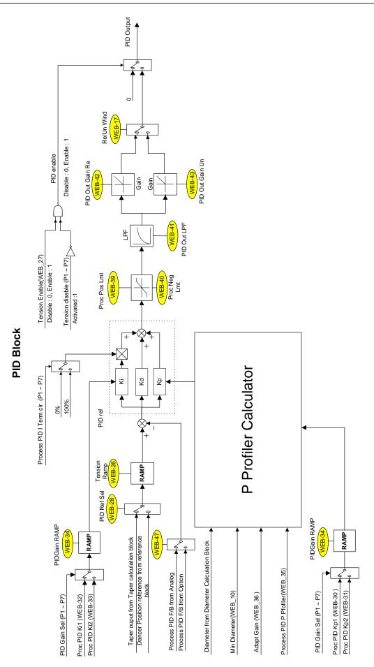
Process PID Block Diagram
