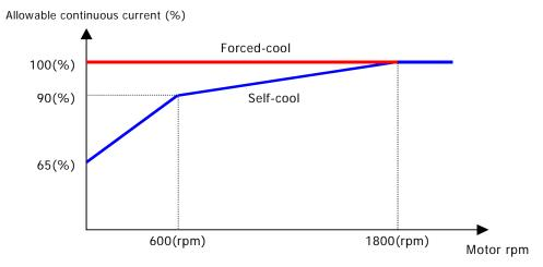
[The characteristic of allowable continuous current with respect to 4 pole, 60Hz motor]
