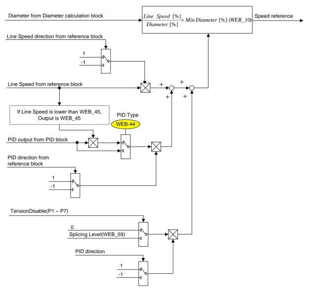
Line Speed Command Block Diagram
