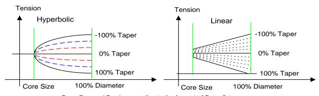
Taper Type and Tension according to the Amount of Taper Set
