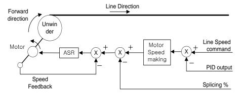
Unwind/Overwind Setting, Roll Rotating Direction in case of Forward Direction Operation
