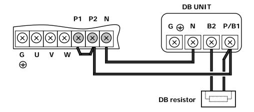
3.3.7 Wiring guide when using both of DC reactor (Option) and DB Unit(option) (30kW and higher) (AC power input: 30kW and higher)
