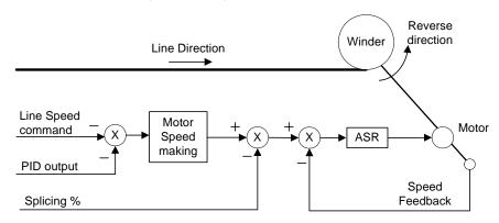
Figure 2. Roll Rotating Direction at the time of Unwind/Overwind Setting, Forward Direction Operation Command
