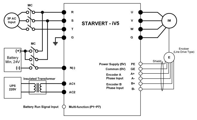
Note) ●: Main circuit, O: Control circuit
