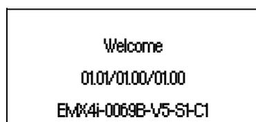
Software versions: user interface, motor control, remote keypad
