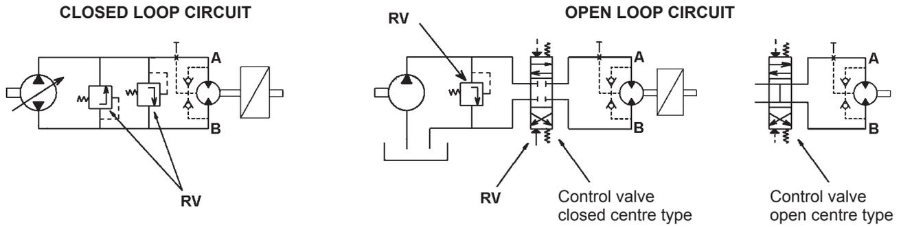
**RV** = Max pressure valve set to a  $p_{RV} < p_{max}$
