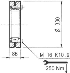
Material: Case hardening steel 18NiCrMo5 UNI 5331 must be case hardened 50-55 HRC
