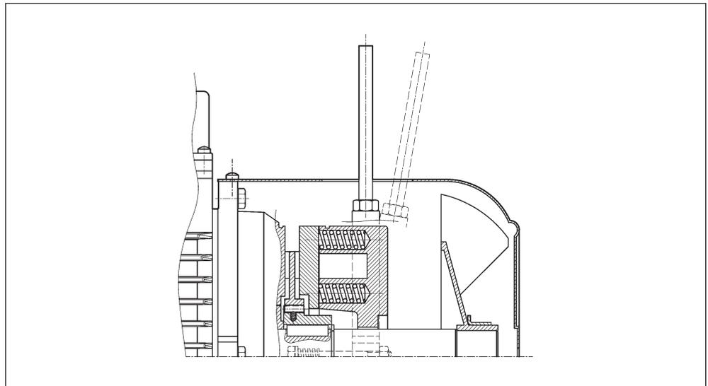
On brake motors type FD, if the option RM is specified, the release device may be locked in the "release" position by tightening the lever until its end becomes engaged with a brake housing projection. The availability for the various disengagement devices is charted here below:
