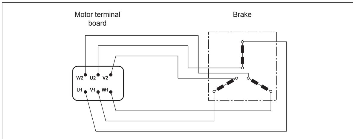
Switch-pole motors and, at request, single-pole motors with separate power supply are equipped with an auxiliary terminal board with 6 terminals for brake connection.
