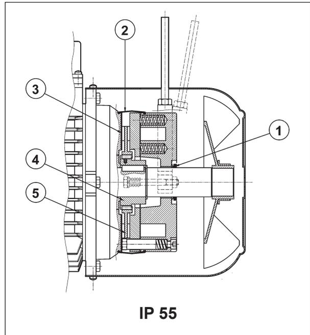
**Direct current** toroidal-coil electromagnetic brake bolted onto motor shield. Preloading springs provide axial positioning of magnet body.
