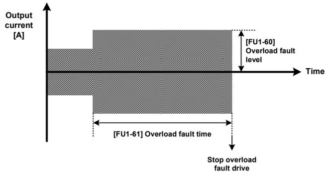
Figure 6-16 Overload Fault
