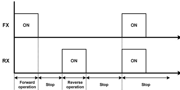
Figure 6-4 Terminal block operation (Fx/Rx-1)
