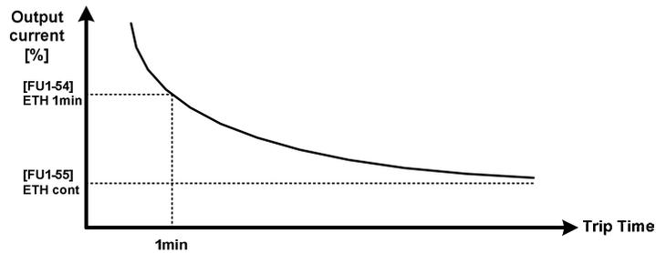
Figure 6-18 Characteristic curve of the electronic thermal level
