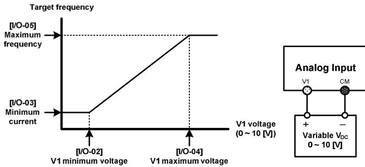
Figure 6-1 Frequency commands by voltage and wiring diagram
