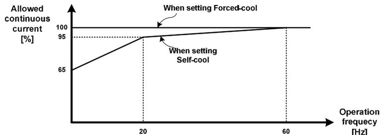
Figure 6-17 Characteristics of permissible continuous current reduction by frequency
