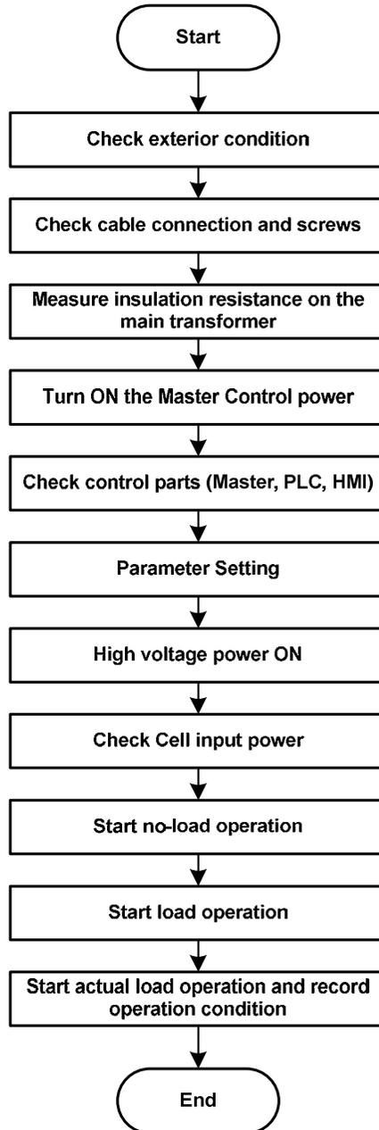
Figure 4-1 LSMV Test Operation Order
