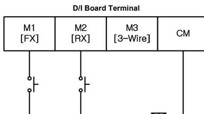
Figure 6-20 Example of a 3-Wire Operation Connection
