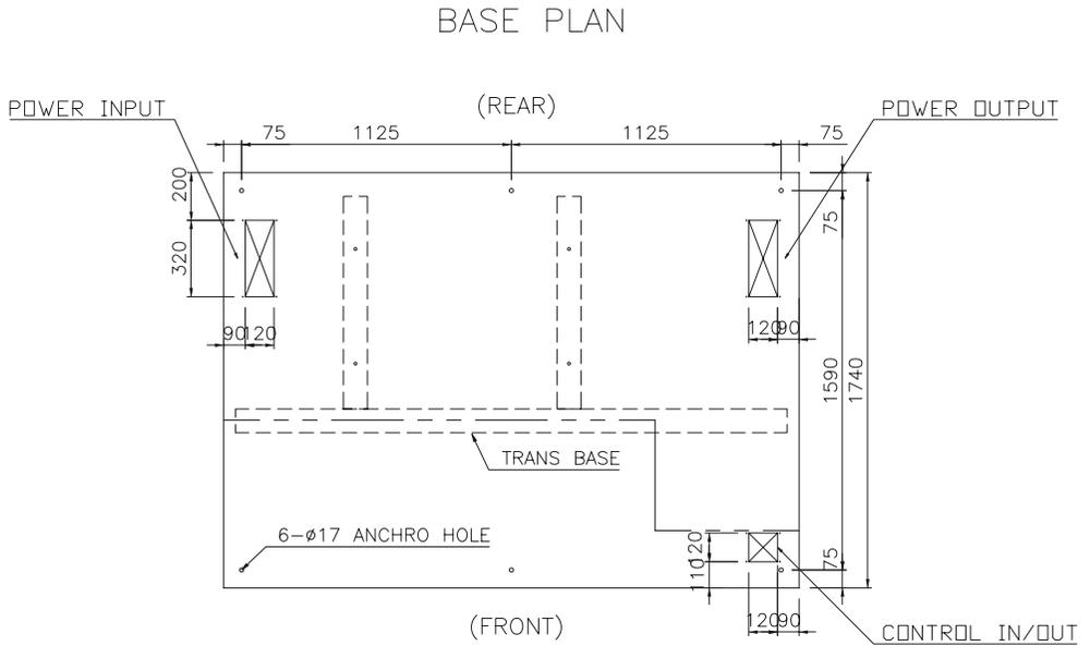
**Figure 1-9 LSMV-066S600-G1 (Type A) Base Plan**
