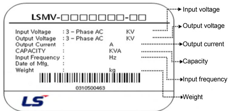
Figure 1-1 Standard Plate Format
