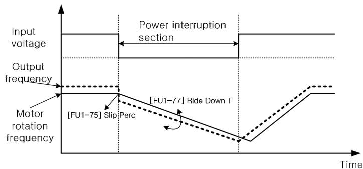
Figure 6-20 Continuous Operation Feature for Instantaneous Power Interruption
