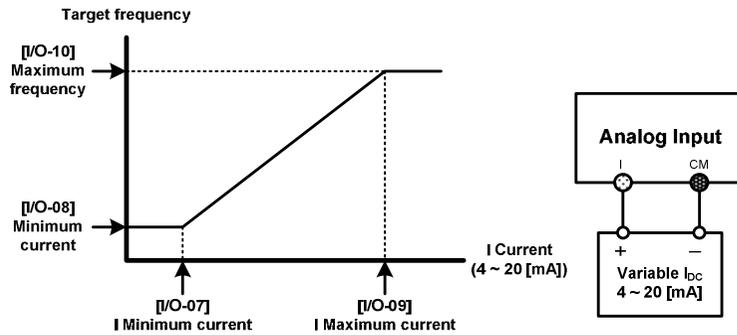
Figure 6-2 Frequency commands by current
