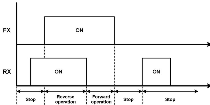
Figure 6-5 Terminal block operation (Fx/Rx-2)
