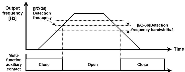
Figure 6-19 Frequency Detection (FDT-5)
