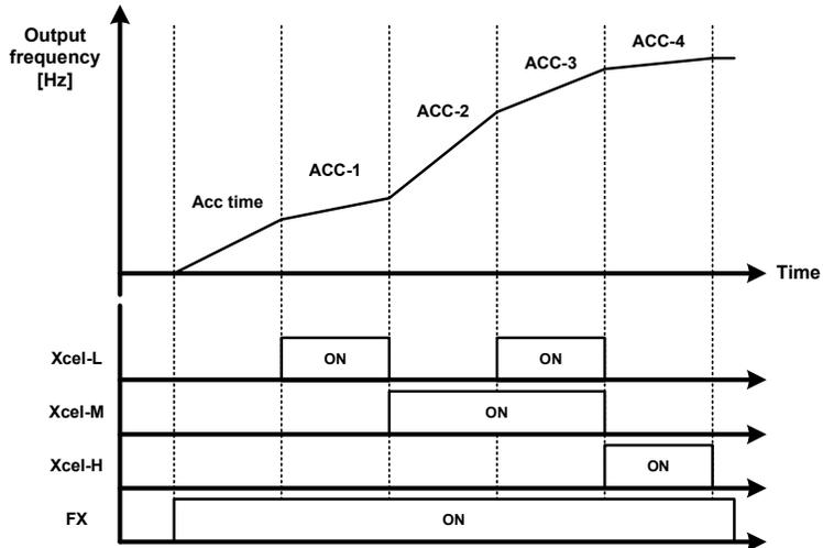
Figure 6-24 Applying Accel/Decel Time
