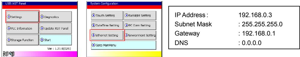
Figure 11-35 Enter HMI IP
