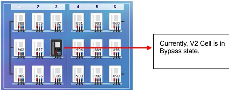
Figure 11-45 Cell Bypass
