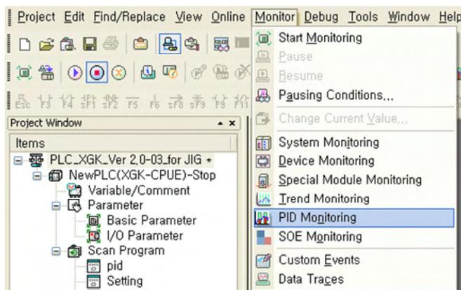
Figure 11-12 Launch PID Monitoring
