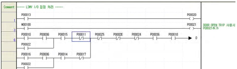
Figure 11-28 Processing Input/Output Contact
