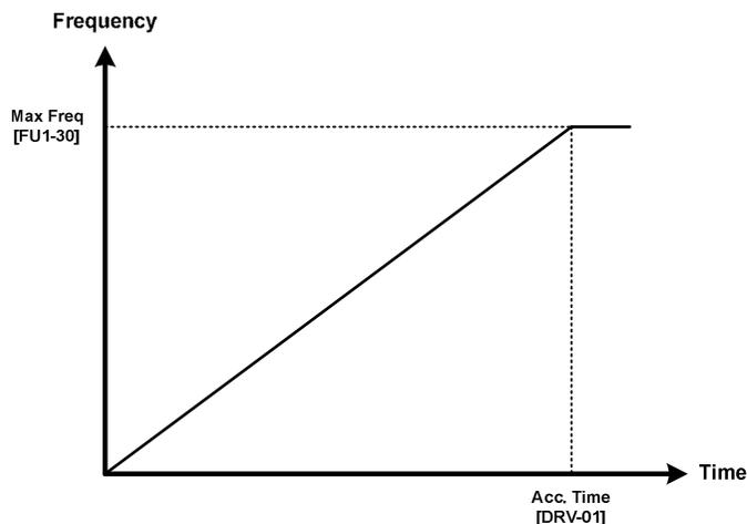
Figure 6-6 Acceleration Pattern during Accel Start (Linear)
