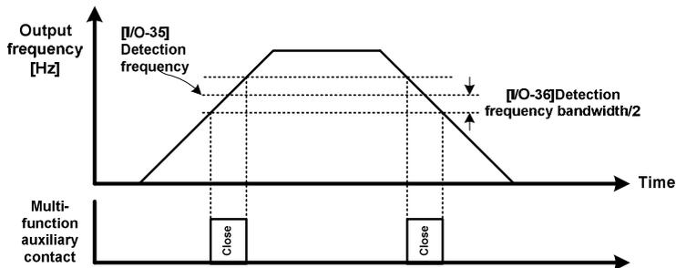
Figure 6-17 Frequency Detection (FDT-3)
