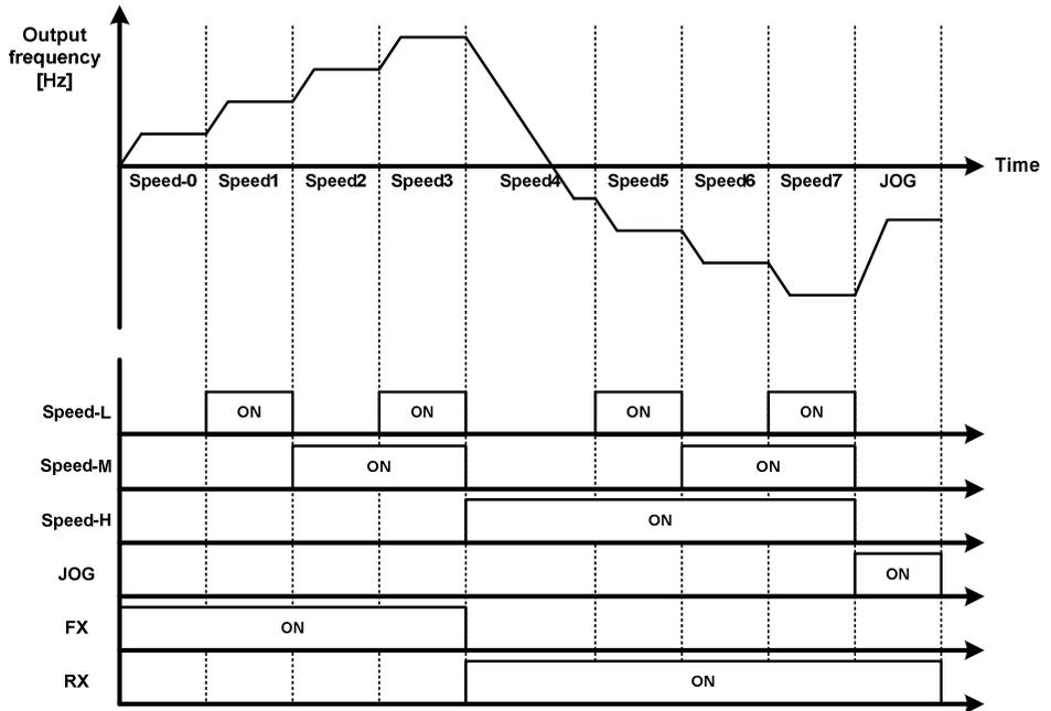
Figure 6-23 Jog and multi-step speed operation
