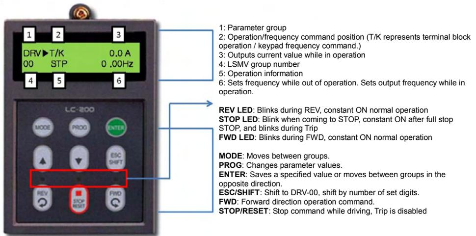
Figure 3-1 Keypad Configuration and Functions
