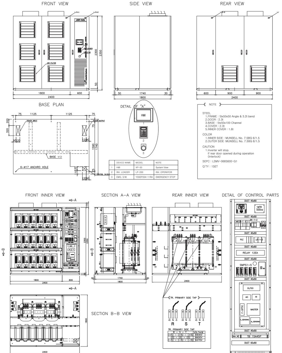
Figure 1-3 LSMV-066F600-G1 Exterior and Interior Block Diagram
