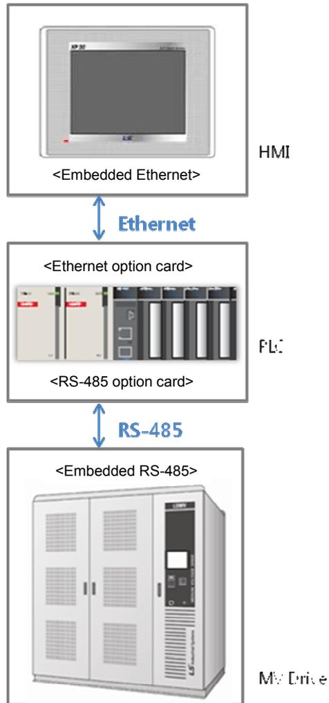
Figure 11-1 HMI Configuration
