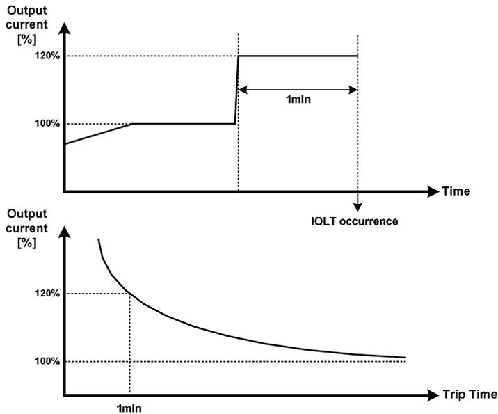
Figure 6-15 Drive Overload (Inv. OLT) Fault
