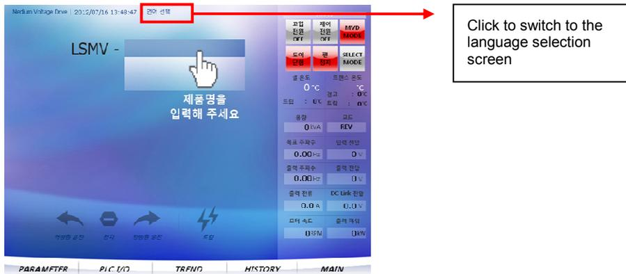
Figure 11-38 HMI Main Screen
