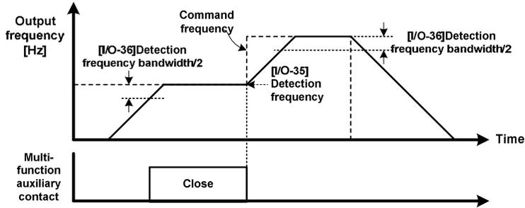
Figure 6-16 Frequency Detection (FDT-2)
