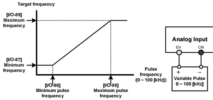
Figure 6-3 Frequency commands via pulse
