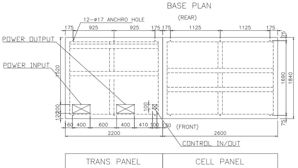
**Figure 1-10 LSMV-066S30H-G1 (Type B) Base Plan**
