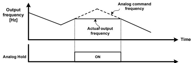
Figure 6-22 Analog Hold Operation
