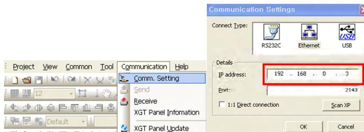
Figure 11-31 HMI IP Address
