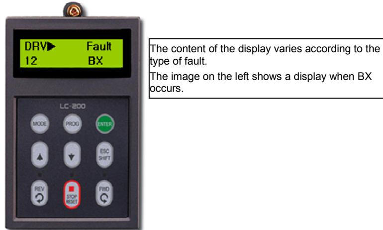
Figure 4-2 Keypad Display When a Fault Occurs
