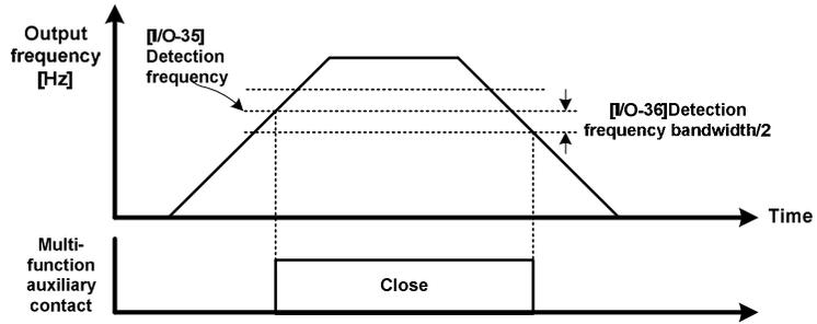
Figure 6-18 Frequency Detection (FDT-4)
