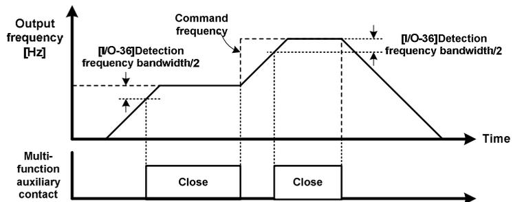
Figure 6-15 Frequency Detection (FDT-1)
