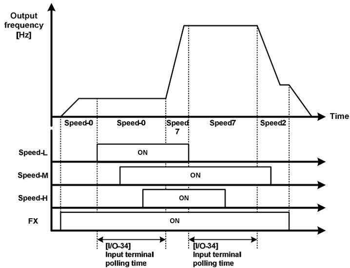
Figure 6-25 Change of allowed time for input
