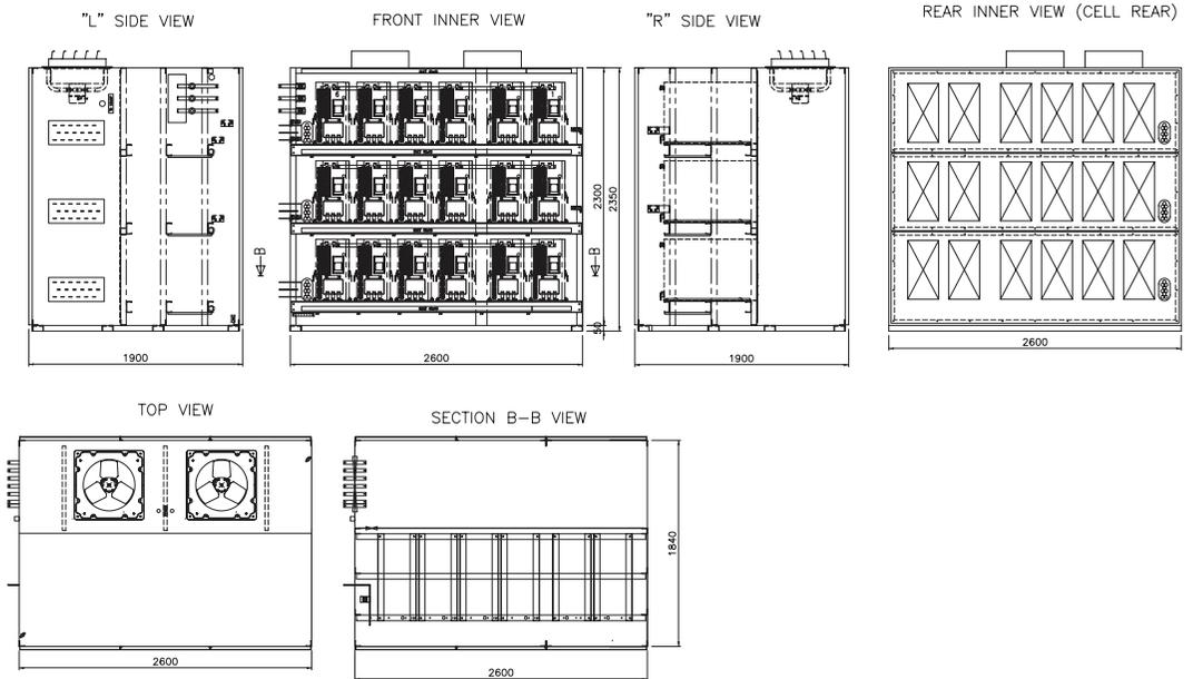
Figure 1-4 LSMV-066S30H Exterior and Interior Block Diagram
