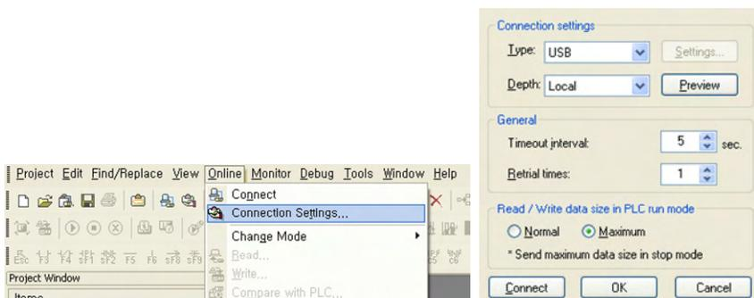
Figure 11-10 Computer and PLC Connection
