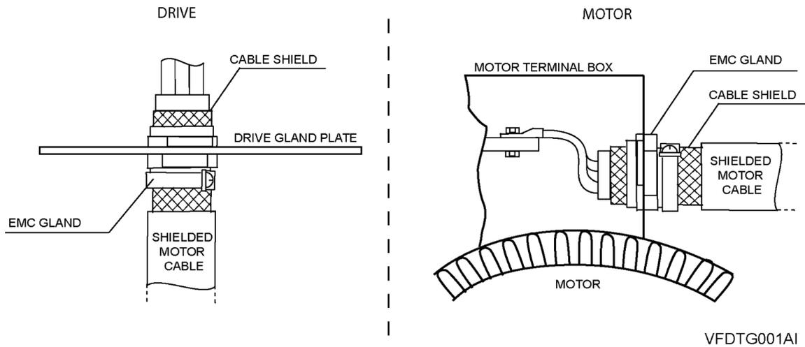
Correct output motor cables shield bonding
