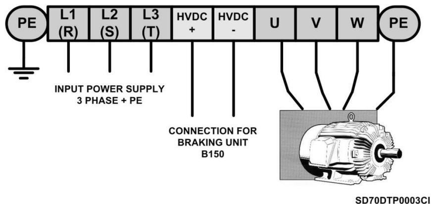
The input terminals L1, L2, L3 and PE (drive power supply), output terminals U, V, W and PE (motor power supply) must be introduced through the metal plates situated in the bottom part of the cabinet. Do not drill or mechanize the vents. Otherwise, the drive could reduce its cooling capacity.
