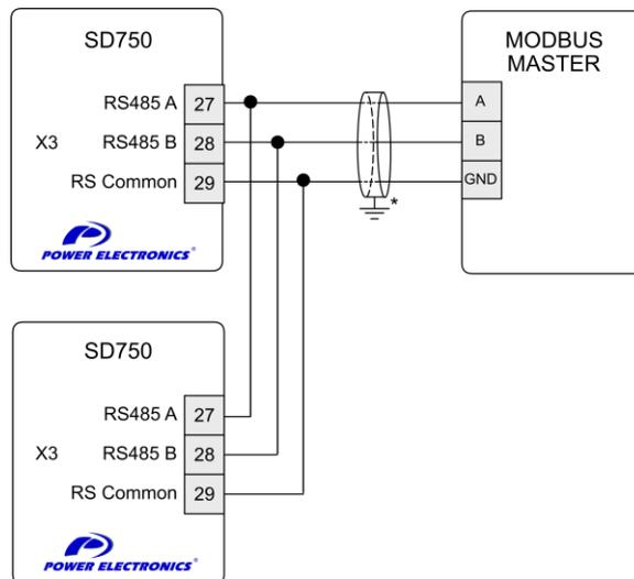
\* Screen connection must be performed on the side of the Modbus master or on the other side depending on the installation.
