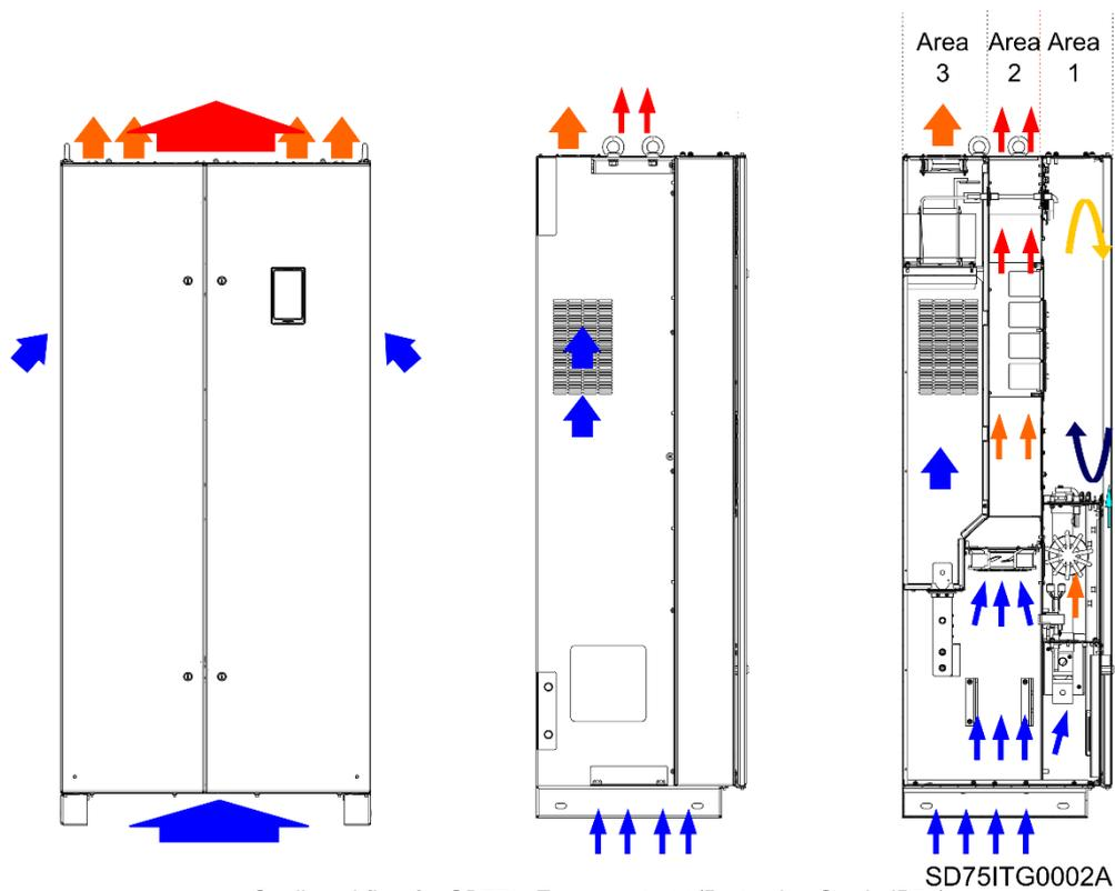
Cooling airflow for SD750. Frames 4 to 11(Protection Grade IP54).
